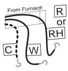
**STEP 1 -** Connect the **R** (or RH) wire to the **RH** terminal on the thermostat.
