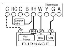
**STEP 2 -** Connect the **W** wire to the **W** terminal on the thermostat.
