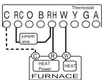
**STEP 2 -** Connect the **W** wire to the **W** terminal on the thermostat.
