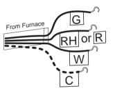
**STEP 1 -** Connect the **R** (or RH) wire to the **RH** terminal on the thermostat. This connects to the Heater Power .
