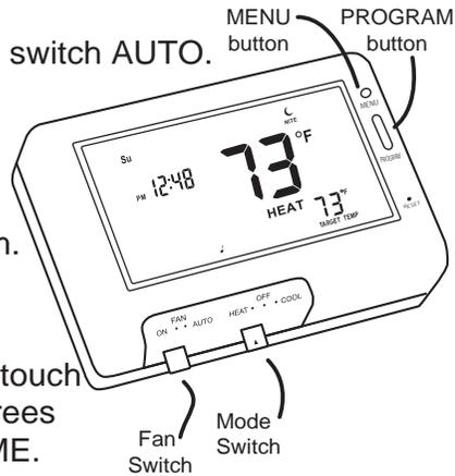
To check Fan: (If you connected the G wire - fan relay)
