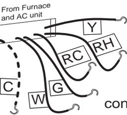
**STEP 1 -** Remove the red Jumper wire.
