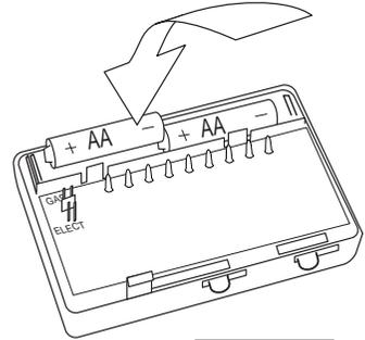
NOTE: Replace the batteries when this LOW battery **LOWBATT** indicator appears on the display or once a year. When replacing batteries, you have approximately one minute before your custom program is lost.
