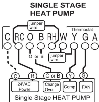
**NOTE:** Wires marked with the dotted line are optional.
