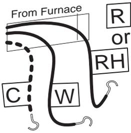
**STEP 1** - Connect the **R** (or RH) wire to the **RH** terminal on the thermostat. This connects the Heater Power to the thermostat.
