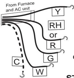
**STEP 1 -** Connect the **Y** wire to the **Y** terminal on the thermostat. This connects to the Cooler compressor.
