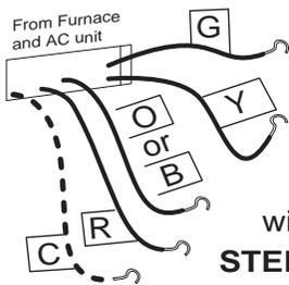
**STEP 1** - Connect the **G** wire to the **G** terminal on the thermostat.
